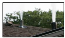
non-toxic mineral oil based smoke that workers will blow into the sewer system. During the test, you can expect to see smoke escaping through vent stacks on the roof of your home and neighboring homes (see picture to left), indicating the building's plumbing was properly installed. It is important to note that test smoke emitting from roof vents does NOT indicate the home is
